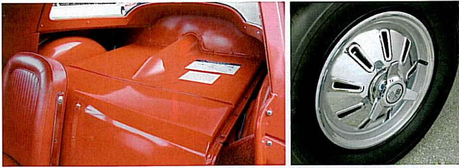
Above left: Fitting the optional 36.5-gallon fuel tank necessitated unique trim. Above right: Optional alloy wheel with knock-off. Below: There's no radio in this Corvette; it is also devoid of air-conditioning and has no heater.
