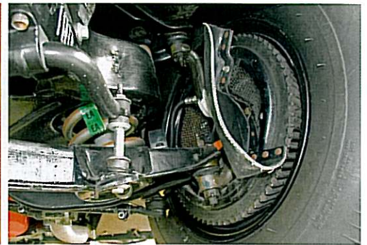
Above right: Drum brakes feature wide sintered metallic linings and "elephant ear" air scoops to aid cooling. Below: Displacing 327 cubic inches and utilizing mechanical fuel injection, this L84 V8 generates 375 bhp.
