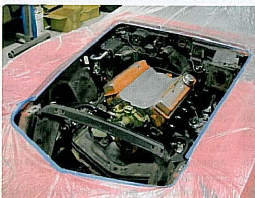
Above: Below the tuned-port fuel injection and shiny new valve covers lays the original 327 small-block V8. Below, left to right: The engine is stripped down and ready to be updated at Carr's Corvettes and Customs; the dash got the modernization treatment, as well. Bottom: Mostly stock interior features iPod-ready radio.
